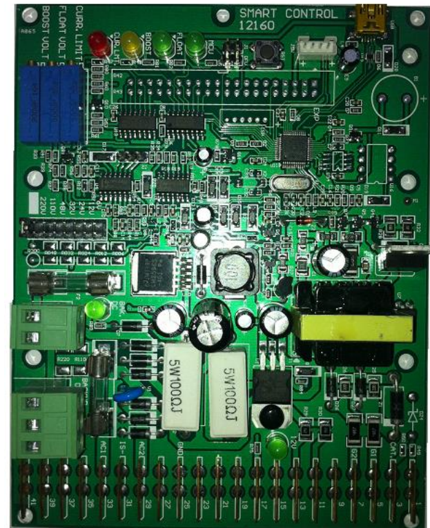
Smart 1 Phase control Card P/N: Smart 12160
